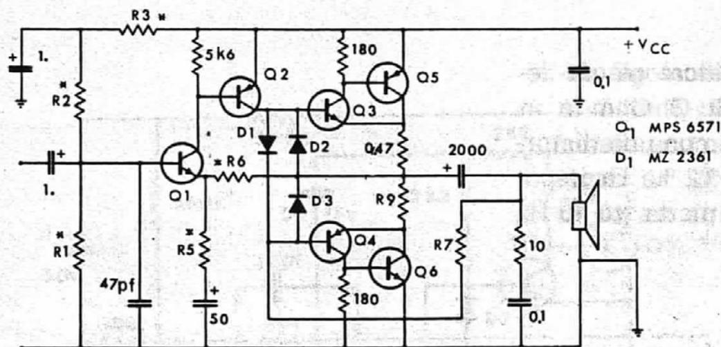
Resistors : 1/2W 10% or 5% (\*) Tolerance
